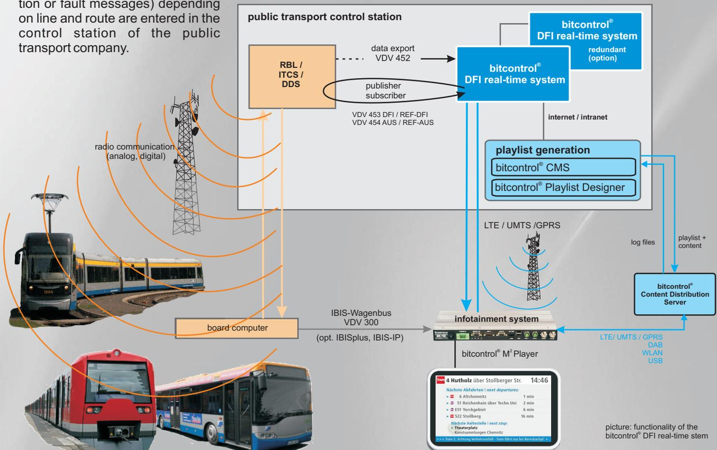
picture: functionality of the bitcontrol® DFI real-time stem
